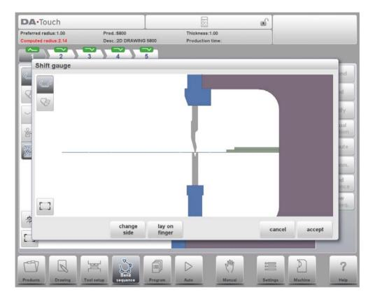
The fingers can be moved by means of the different available functions.
