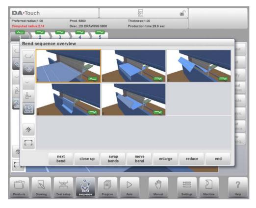
This option can be called at any time after the first unbend has been made. The graphical overview displays the determined bends as well as the not yet determined bends (question mark sign).
