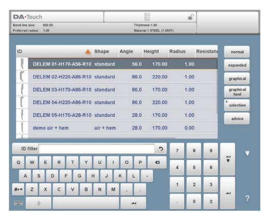
If only a part of the tool ID is typed, the control automatically offers a list of tools with the typed characters. This is a filtering function.
