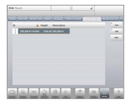
The shapes of your machine are drawn in the same way as for the punches and dies. Like with the tools the right hand side of the drawing is the back gauge position of the machine. To have a more detailed view in the library tab, tap View and use Graphical.
