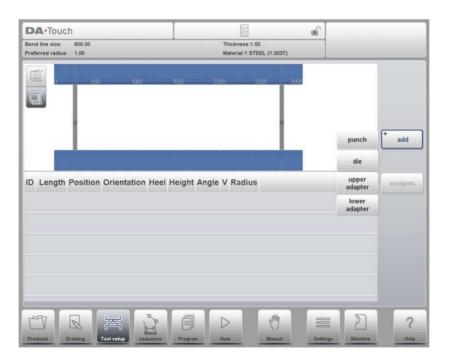
When a tool has been chosen (e.g. a punch), it is placed in the machine with maximum available length.
