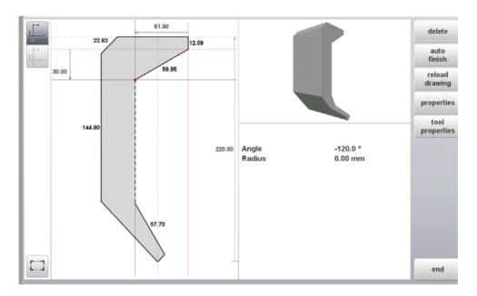
• To your convenience that help lines can be switched off. Giving a non disturbed view to what you have drawn. In case the control is using mount points in the tool details, the mount points can be toggled with the drawing. This prevent from accidental non desired changes to either mount point position or shape details.
