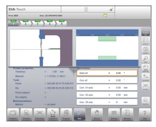
Both lower columns can be scrolled to see all data. In the graphical view quadrant zoom, pan and rotate can be used to view the bend position in the machine.
