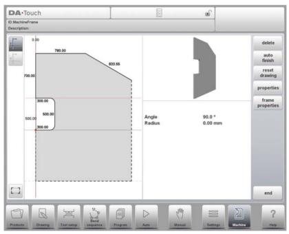
When using this graphical programming function it replaces the parameterized frame programming.
