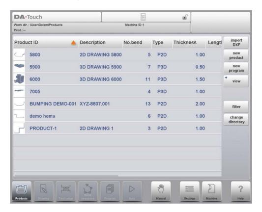
When a new product drawing is started a screen with general product properties appears. First these properties, general data, should be set before starting with the product drawing.
