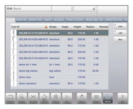
Navigation through the tabs can be done by just tapping them and selecting the required item to adjust. Since there can be more tabs than the screen can show in one view, dragging the tabs in horizontal direction enables to view and select all available tabs.
