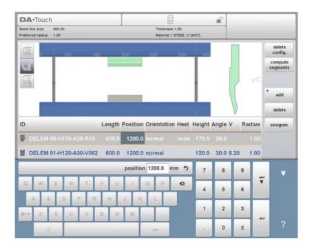
When dragging tools, or tool stations, the snapping function will assist in aligning the upper tool with the lower tool at left or right, or the tools or toolstations with the middle of the machine. At the time tools are within the snapping zone, a red line will appear indicating that release will help positioning towards the indicated edge or position.
