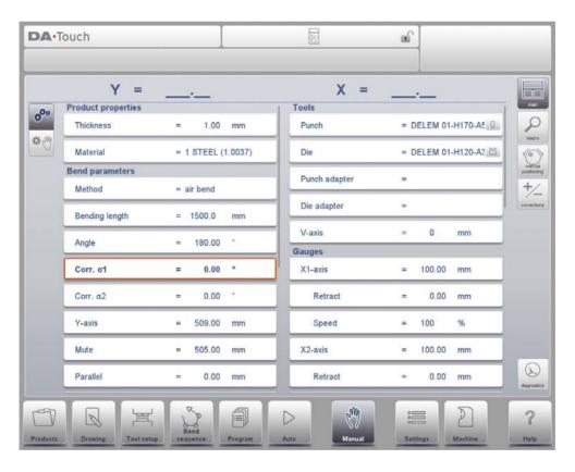
Turn Punch can be used to turn around the applied tool (back to front). When this is done, and active, the indicator is shown behind the punch or die.
