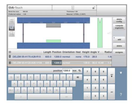
The tool set-up can be modified with the available functions or by changing a value in the list view. Punches and dies can be added or deleted, the existing tools can be moved to a different position, their length can be modified, the orientation can be changed (i.e. the tool can be turned around) and heel types can be changed.
