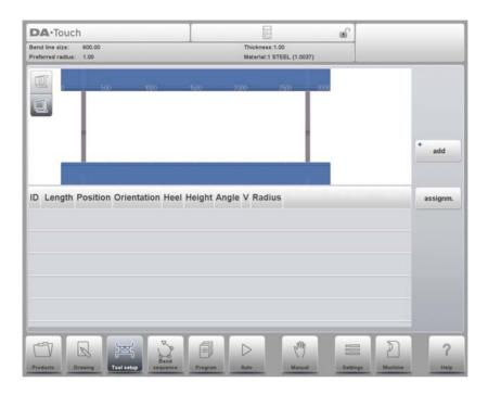
Select Add to add a tool to the configuration; punch, die or adapter (if enabled).
