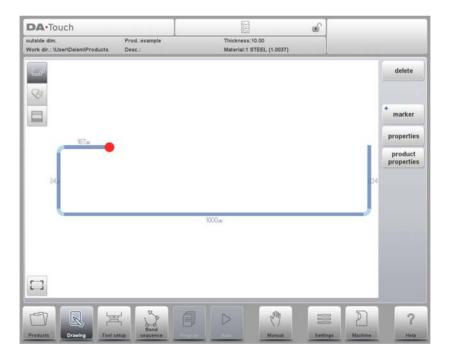
When the product drawing is finished it is possible to navigate to the next step in the programming process; to determine first the Tool Setup and after the Bend Sequence.
