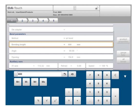
In case calculations should use parameter values as an input, and results as an output, one can switch to the calculator from the parameter entry. This will bring the parameter value to the calculator, and the result back to the input line.
