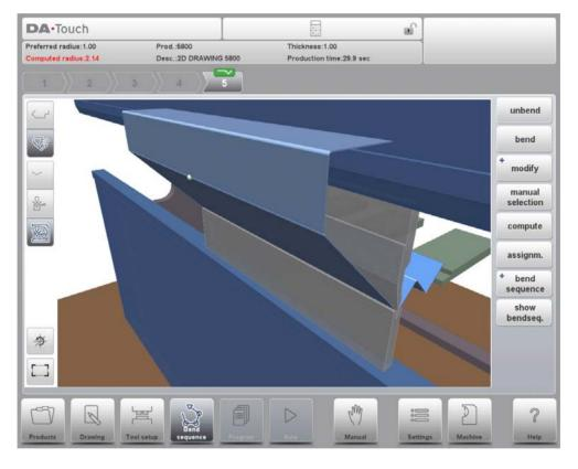
The bendsequence determination can be realised by automatic calculation starting with the bent product. It is also possible determining the sequence manually starting with the flat product, not using the automatic calculation.
