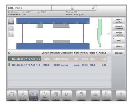
Segments can be changed within the segmentation view. The available segments in stock are not taken into account at that time. With a renewed segmentation this can be verified.
