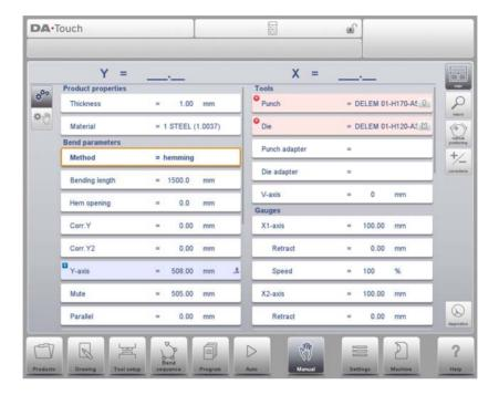
When an information symbol is shown with parameters after an editted value, this parameters was changed due to the last changed input.
