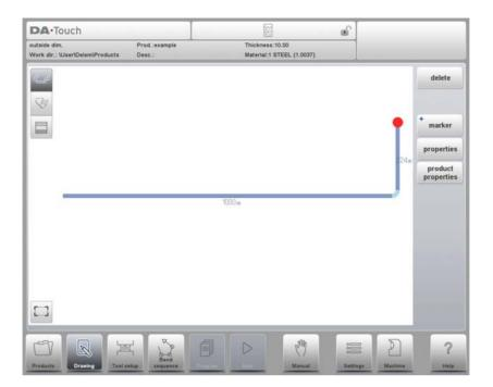
The currently active element (line or angle) is highlighted. In a product drawing you can program up to a maximum of 99 bends per product (graphical programming).
