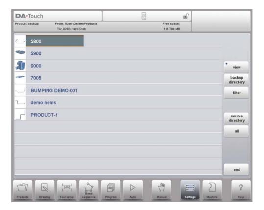
In the backup screen the products in the selected directory are shown. Basic functions to change the view can be chosen similarly to the Products mode. This enables to easily find the required products to be backupped.
