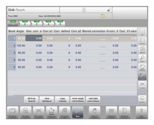
The column 'Stored correction' is only available when the Angle correction database has been activated. When activated, the column 'Stored correction' shows for each bend the correction value that is present in the database. A blank entry in this column means the database does not have a correction value for this type of bend. When a new correction is entered, it will be copied to the database automatically.
