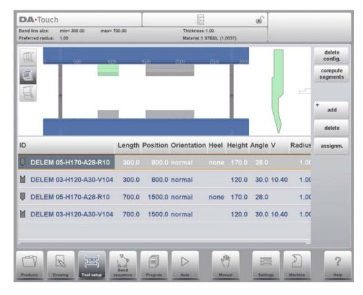
In below paragraph the functionality for segmentation is explained, including the use of the three views on the tool setup. Next to the Tool Setup screen the ability to have segmentation features available is depending on the programmed segments for each tool. This programming can be done in Machine mode under the Punches and Bottom dies libraries. More on programming of segments in the Tool library can be found at the end of this paragraph.
