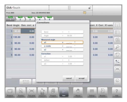
From the programmed value the control will determine a correction. The proposed result can be seen in the window itself. In the top of the window the programmed angle is shown, in the bottom of the window the resulting corrections are shown. When selecting accept, these values will be transferred to the main corrections screen.
