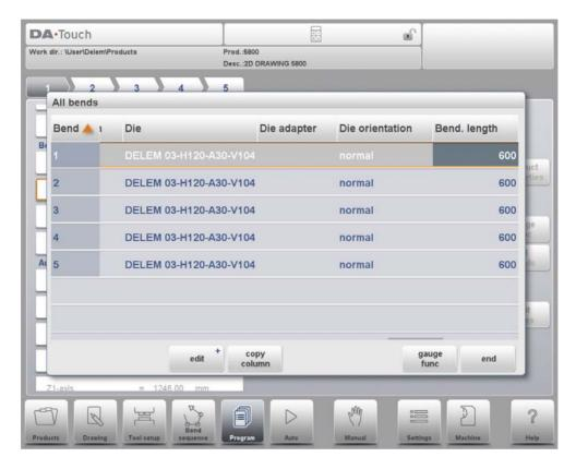
Specific bend can be selected on the screen by putting the highlighted bar on that bend, then selecting END.
