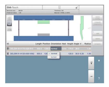
After a tool is placed, the tool ID can be changed by selecting the Punch ID in the screen and tapping on the List view.
