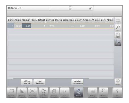
The programmed corrections can be verified here similarly to the corrections in Automode. Entries in the correction database and for initial correction can also be monitored in this screen. Since these are of significant influence on the bend result, access to the database can be used to modify. This can also be usefull while finding appropriate corrections with testbending and storing the found results in the database.
