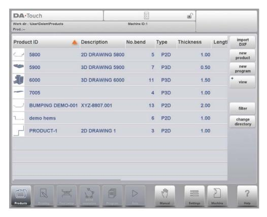
Depending on the navigation button which is active, the screen will differ. The above main screen will appear having the Products function active.
