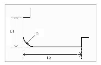
Lengths L1 and L2 must be equal or bigger than the radius R.
