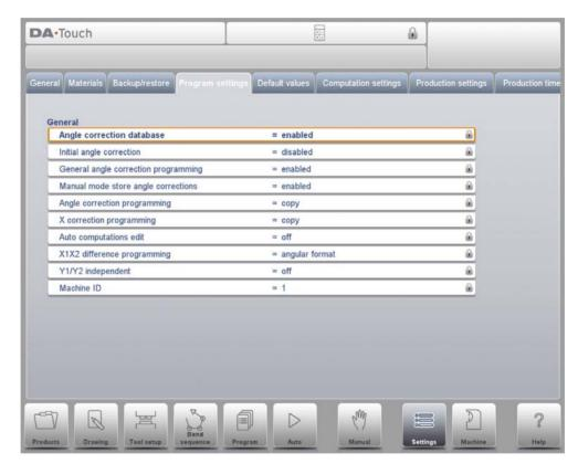
Lock symbols when Program Lock is active will also appear behind parameters to show the lock is active and modification is not possible.
