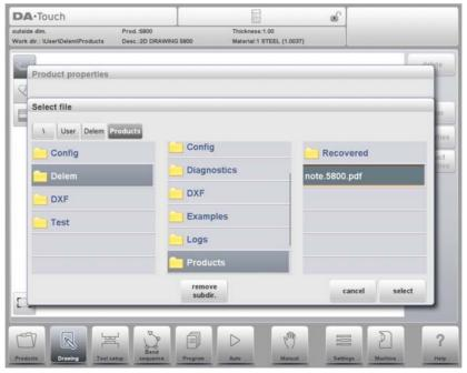
When solely a PDF file is attached without a textual note, the PDF will be shown instantaneously when the user presses the Notes indicator in Auto mode.
