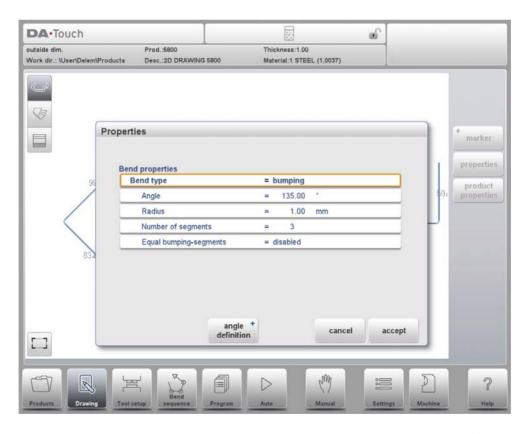
If a tool with large radius is not available, the bumping method can be chosen. With this method, a large radius in a product is obtained by a series of slight bends in succession.
