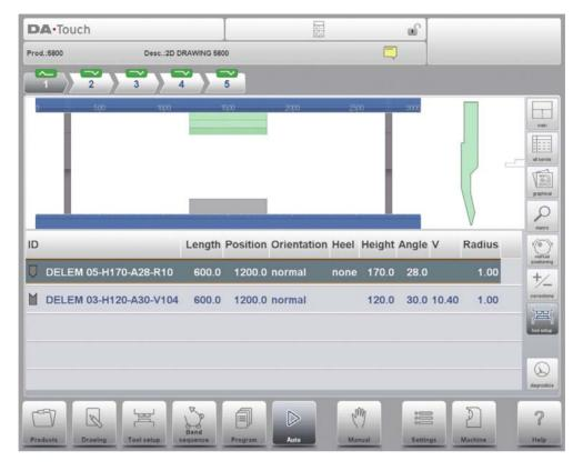
In this tool setup view mode no changes can be made to the actual setup. If this is required one has to switch to the Tool Setup menu, outside Auto mode.
