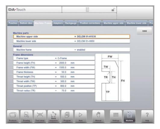
The tabs can easily be selected by just tapping them. When a tab is not completely visible or not visible at all, just by dragging the tab row horizontally, the desired tab can be "pulled" in sight and be selected.
