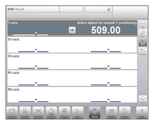
Within this mode, any of the shown axes can be moved by turning the hand wheel. The procedure for moving the axis depends on the axis you wish to move.
