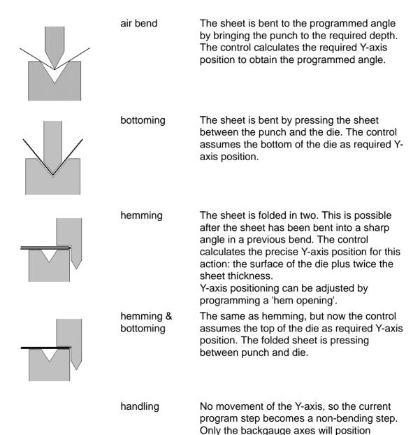
according to the programmed values, e.g. in order to enable handling of the product. An external step change (C-input) is required.
