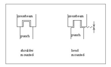
If 'shoulder mounted' is chosen, the Y-axis position is calculated from the standard tool height. This is the default setting.
