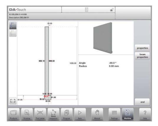
After giving in the base parameters for the specific machine part, the drawing editor appears. Similar to drawing of tools, also the details of the machine parts can be drawn. Either by tapping and sketching or by giving in the length of sides and pointing the direction of the next side.
