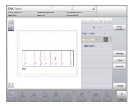
For bendlines, lines as well as texts can be checked. The text near the line indicates its angle value or radius or if it is a hemming. When assigning text to bendlines, the import will use this. For countour lines text information is not applicable.
