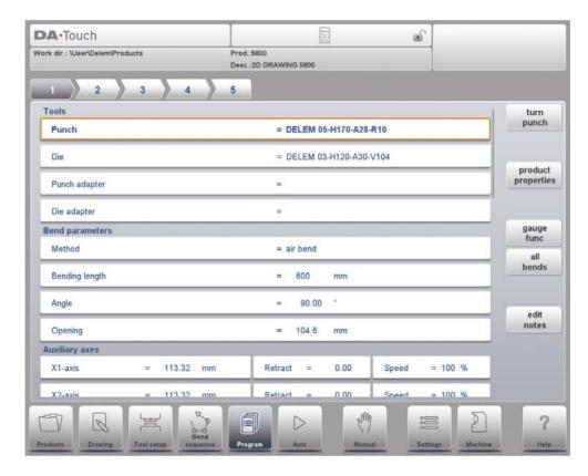
To edit an existing CNC program, select a product in the Products overview and select the navigation button Program. When starting a new program, select New Program and after giving in the main product properties, the system will automatically switch to Program.
