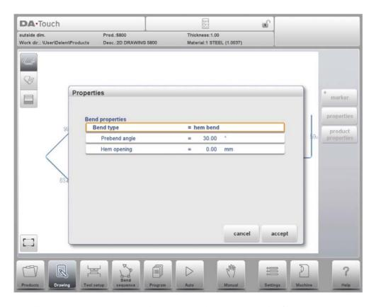
It is also possible to create a hem bend by placing the cursor on the flange end where the hem bend is required and select properties. In this way the pop-up window will appear with an extra parameter to fill-out.
