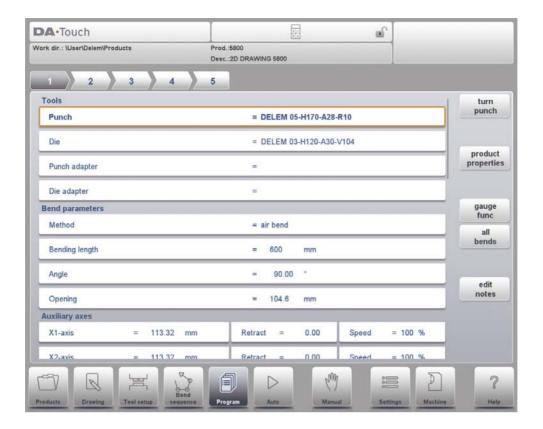
The bend selector in the top of the screen can be used to navigate thru the bends. The indicated bends can be tapped to easily select the desired bend data.
