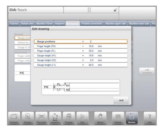
The following parameters describe the dimensions of the backgauge and the lay-on positions. The number of parameters that has to be programmed depends on the number of gauge positions. If more gauge positions are programmed, more parameters are offered. The illustration at the bottom of the screen will change according to the number of gauge positions.
