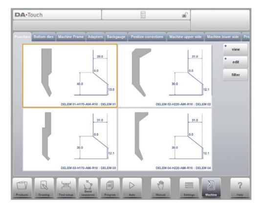
In Graphical Heel the geometry of the tools is shown as well as the heel properties.
