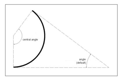
To apply the bumping method, the following parameters must be programmed:
