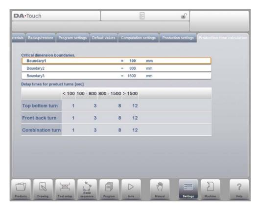
The parameters on this page are used to calculate the production time for a product in the bend sequence computation process . This production time depends on the positioning speed of the axes and the product handling times. The positioning speed is depending on machine settings.
