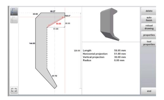
Help lines are provided to measure inter point distances and also enable to change the
