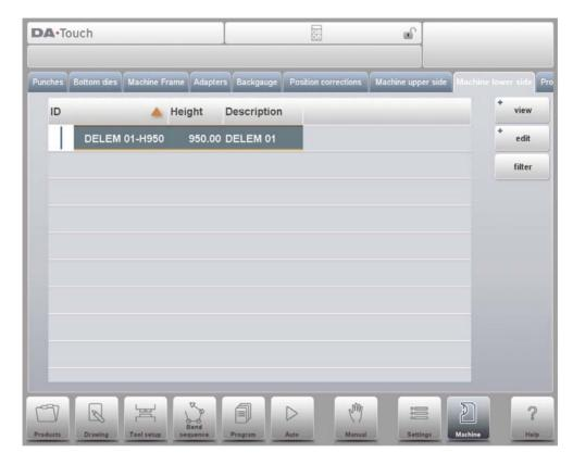
To create a new machine part, tap Edit in the library and subsequently use Add. The control will start by asking for an ID, a description and a height.
