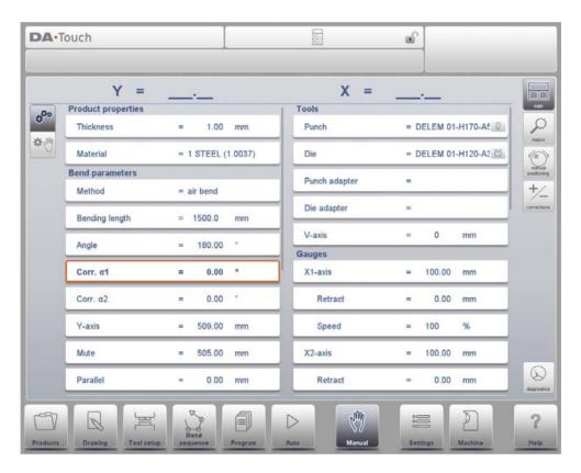
Manual mode is independent from Automatic mode and can be programmed independently of the programs in memory.
