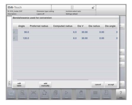
If no bend allowance entry is available, the bend allowance table can be edited directly from this pop-up by tapping the edit table button. The following window will appear and the bend allowance information can be added to the table.
