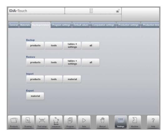
The actual backup directory consists of a device (USB stick, network) and a directory. The choice of devices depends on which devices are connected to the control. If necessary, directories can be created and selected. The backup locations for storage of products and tools are set independently.
