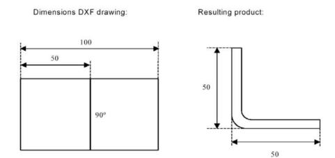
In this example, the length in the original DXF drawing may simply be 100, separated by a bendline. The resulting product will consist of two sides, each with a length of 50. The dimensions are defined as outside dimensions.
