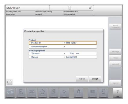
By accepting and closing this window the actual conversion will take place. The result of the conversion is shown in Drawing.
