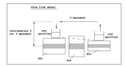
When the back gauge has to move to a different Z-position, it is checked whether the current X-position is safe. We can distinguish the following situations:
