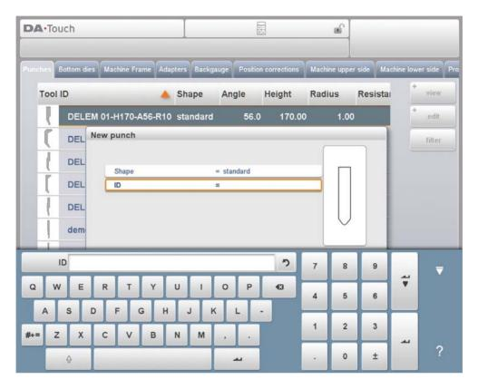
First the basic shape of the punch and its ID must be programmed. After that the shape details must be programmed following the wizard.
