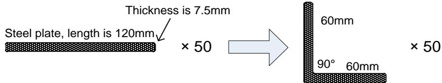
In this example, we can learn a set of the basic data: material is steel; X-axis is 60; bending-angle is 90; thickness is 7.5; stock is 50.
