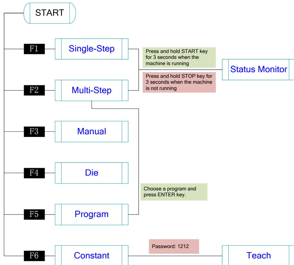
Figure 2-2 Operation flow diagram
