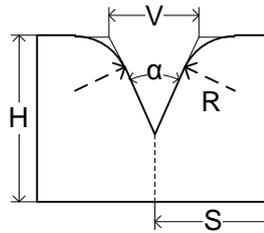
Figure 2-7 The technical parameters diagram of the die
