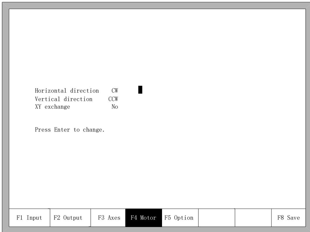
Fig 8.11 Motor direction
