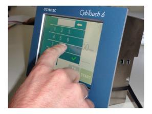
Do not use sharp and/or pointed objects (sheet metal, screwdriver, metal pen ball, etc.) to touch the screen; only use your fingers (with or without gloves on) or a plastic pen. Make sure that your gloves do not have metal particles encrusted in the finger tips as they may also damage the screen.
