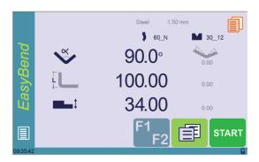
The EasyBend page is used for individual bends, for example when an external worker needs to interrupt production just to make a single bend (usually with the same tools). https://www.machinemfg.com/
