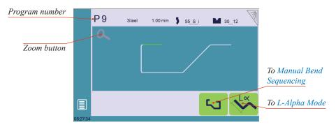
In this mode, the operator can very intuitively draw a profile directly on the screen.
