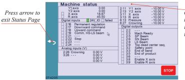
On the upper line, a cycle message may appear indicating the cycle phase the machine is executing
