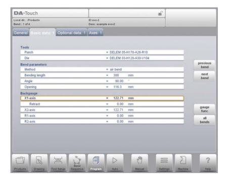
If Gauge Func is pressed, a window appears with several programmable parameters. These parameters serve to program the desired finger positions for a certain bend. The necessary axis positions that are necessary for this bend are calculated from the programmed finger positions
