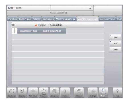
For the lower side of the machine the height is defined from the table surface to the floor level.
