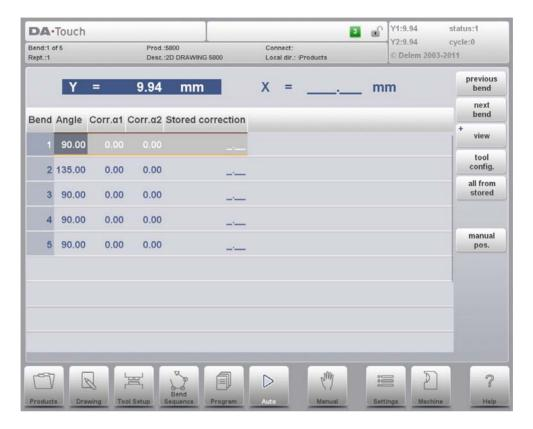
In this window the corrections of all bends are shown. You can browse through all corrections and change them as you see fit. If a correction for 1 is entered then this value is copied to the correction for 2. Different corrections for 2 can be entered in the field itself.
