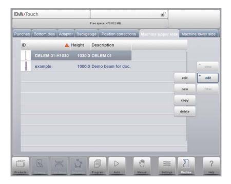
The shapes of your machine are drawn in the same way as for the punches and dies. Like with the tools the right hand side of the drawing is the back gauge position of the machine. To create a new machine part tab Edit in the library and subsequently use Add. The control will start by asking for an ID, description and height.
