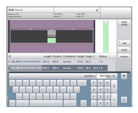
The tool set-up can be modified with the available functions or by changing a value in the list view. Punches and dies can be added or deleted, the existing tools can be moved to a different position, their length can be modified and the orientation can be changed (i.e. the tool can be turned around).
