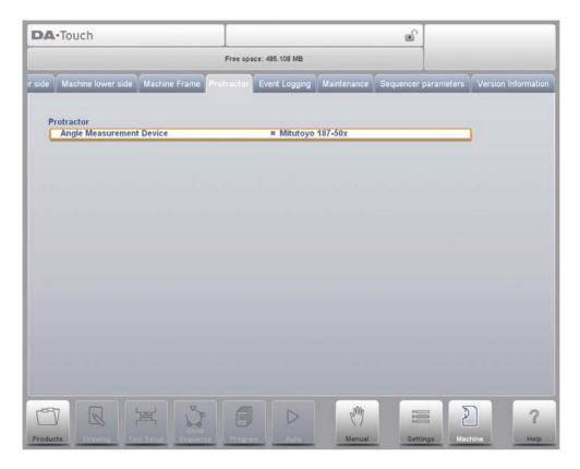
With this parameter you can select a digital angle measuring device when the option OP-W-PROTRACTOR has been installed.
